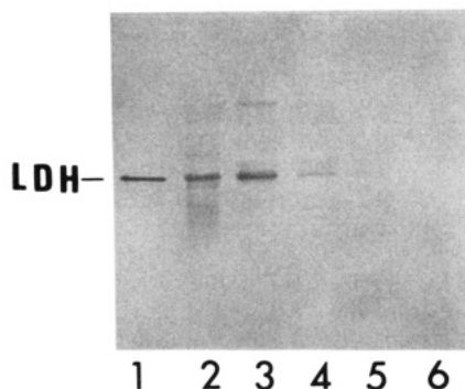
Figure 9. Western blot of isolated turkey muscle LDH and muscle extracts from turkey rolls heated to different end-point temperatures. (Lane 1) Isolated turkey muscle LDH; (lane 2) unheated turkey roll; (lane 3) 68.3 °C; (lane 4) 69.7 °C; (lane 5) 70.9 °C; (lane 6) 72.1 °C. The amounts of protein loaded on the gel lane were 0.07, 1.2, and 20 µg for isolated turkey muscle LDH, unheated turkey roll, and heated turkey rolls, respectively.
